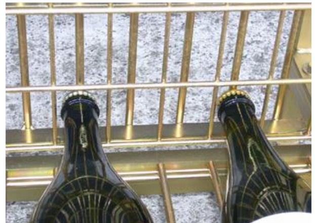
Unique grid system for crown seal location provides support and extra tolerance for diameter variations
